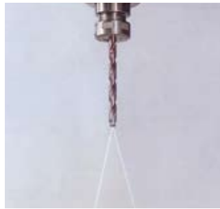
Coolant Through Spindle (CTS) 1.5 MPa CTS used for BT spindle. * Please consult Brother for use of 3 MPa CTS.
