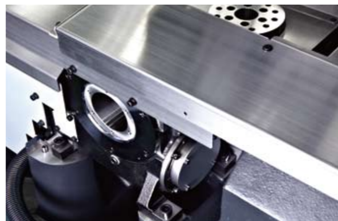
A roller drive mechanism is used for the tilt axis (A-axis). As the index unit is clampless, high-speed and highly accurate indexing is possible.
