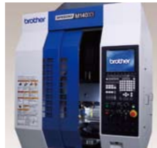
Automatic door (motor-driven) A motor-driven door is used, achieving smooth operation.
