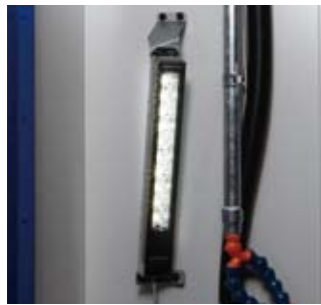
LED type work light (1 or 2 lamps) LED lamps are used to extend lamp life and save energy.
