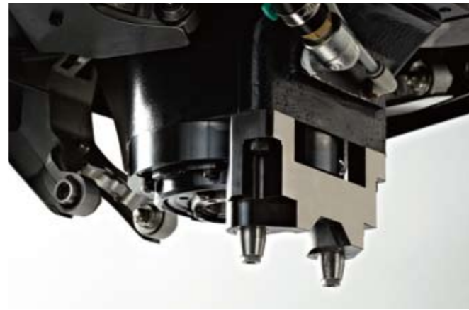
A double plunger lock is used to secure the turning tool to the tool spindle, achieving stable machining.
