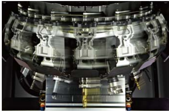
High-speed tool change is possible due to the ATC magazine being mounted around the column. Up to 22 tools can be stored.
