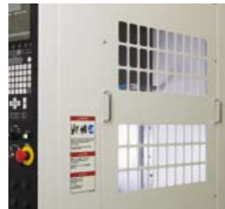
Side cover (transparent board type) External light is drawn in to make the inside of the machine brighter and improve visibility.
