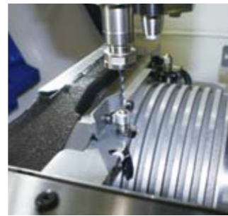
Tool breakage detector (touch type) A touch switch type tool breakage detector is used.
