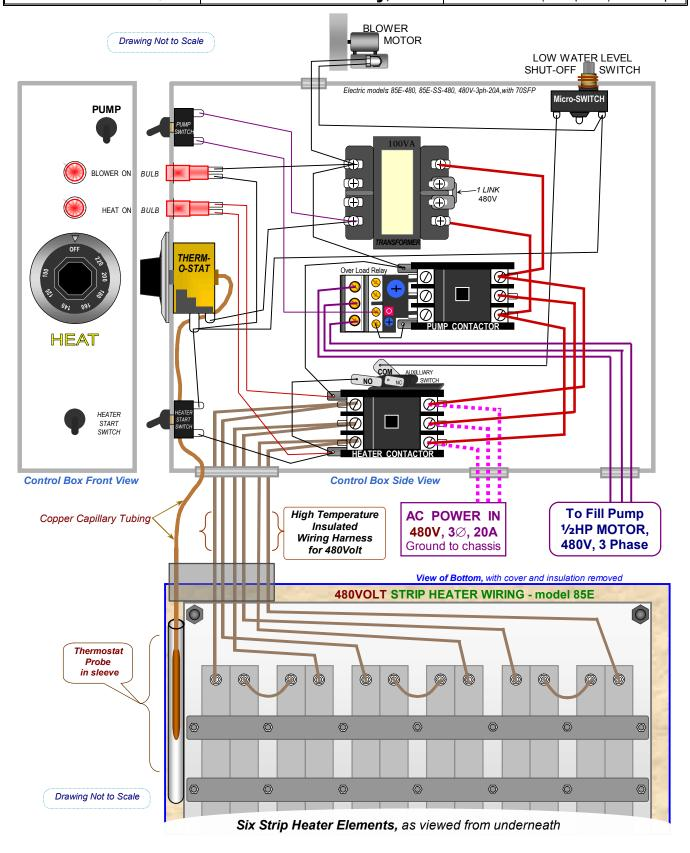
Wiring Diagram for :WATER HEATERmodels:125E-480 and125E-480-SSdwg: WE-125E-480V-3PH-68A-NO-FP-NO-AFS<br/>BC-08-08-2000/ Indeed rev. 09-29-2014EVAPORATORmanufactured 1999 through 2014480V Electric Heated with Optionwith FiLL PUMP only, NO AFS480Volt / 3∅ (three phase) / 34Amps
