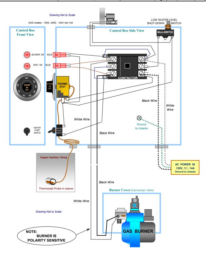
Wiring Diagram for: WATER HEATER models: 375G, 375G-SS
