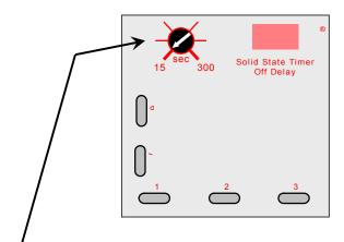
Set slightly LONGER than Countdown Pump Timer cycle. (e.g.: if pump cycle is 13 seconds, set this relay for 15 seconds)
