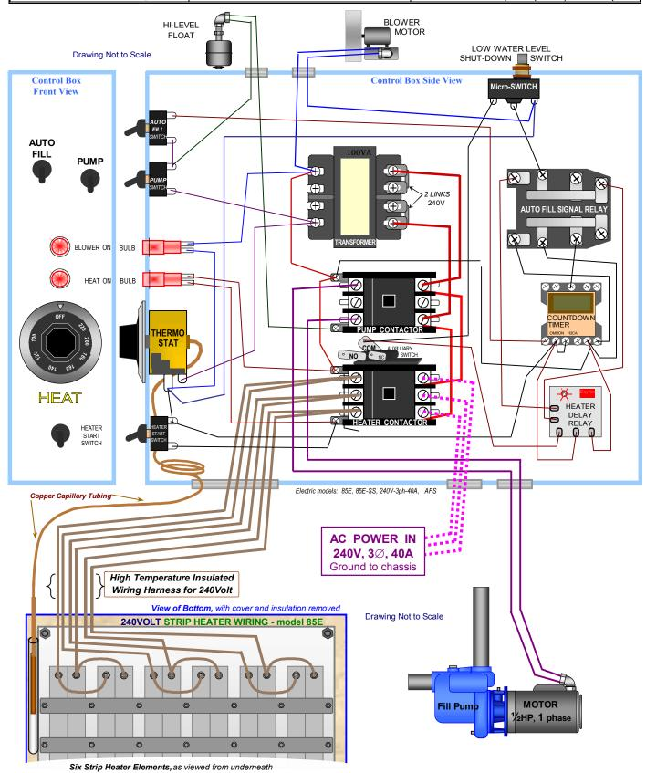
Wiring Diagram for: WATER HEATER EVAPORATOR models: 85E and 85E-SS
