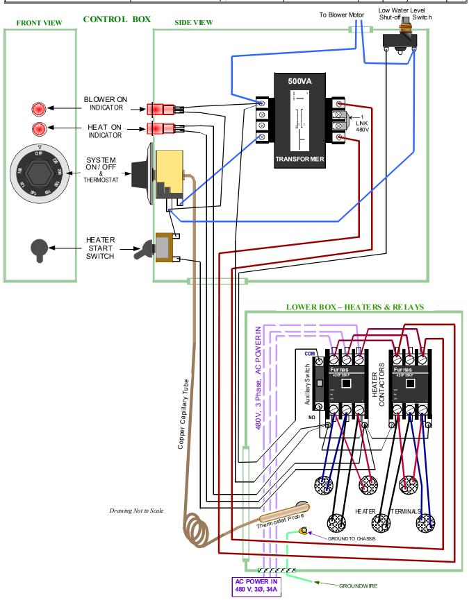
Wiring Diagram for :
