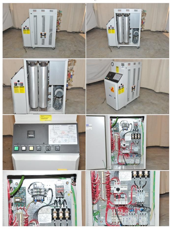
Model # TCO-1 Serial # 37L0533 DWG # 682-92037 - 00 REV E 480 PH 3 VOLTS HERTZ 60 FLA 31 HTR KW 24; 0; 0; 0
