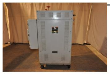
**Description:** Used, AEC Model TDH-5 36 KW Single Zone Portable Hot Oil Process Heater Temperature Control Unit with Cooling Water Circuit For Sale, Features include: Compact Design, Easy-Access Side Panels, , , , , Eurotherm 3216 Controls, Second Hand, DCM-4868
