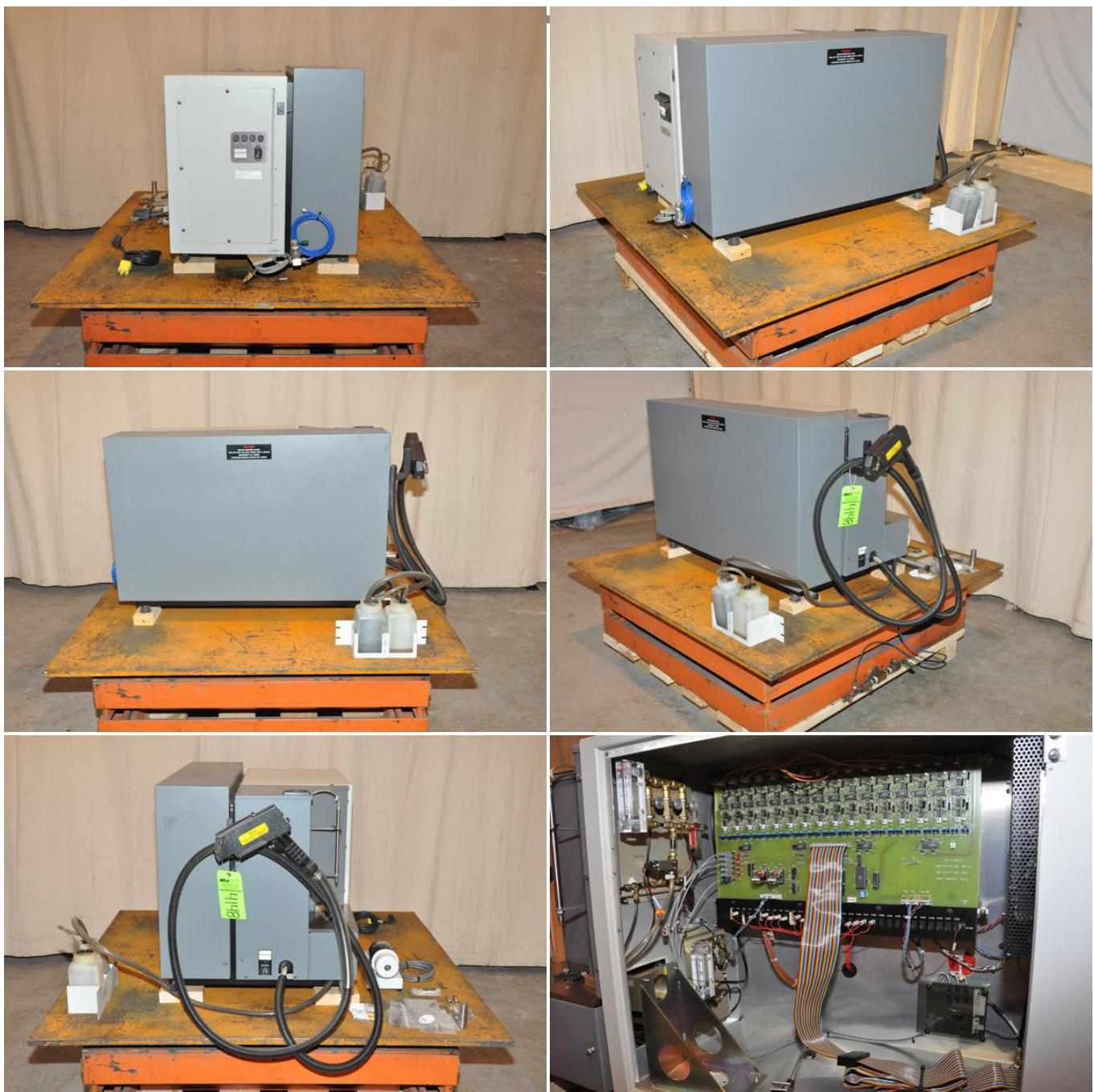
**Description:** Used, Baird Model FoundryMate 16 element Arc/Spark Optical Emission Spectrometry (OES) analyzer Metal Analytic Spectrometer For Sale, Features include: , , , , , Controls, Second Hand, DCM-4148
