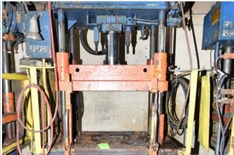
**Description:** Used, B&T Model Greenlee Rapid-Press 20 20 U.S. Ton Four Column (Post) Vertical Hydraulic Die Casting Trim Press For Sale, Features include: Dual Pull-Out Bar Operation, Drill &Tapped Base and Moving Platen, Relay Controls, , , , , Relay Controls, Second Hand, DCM-4853
