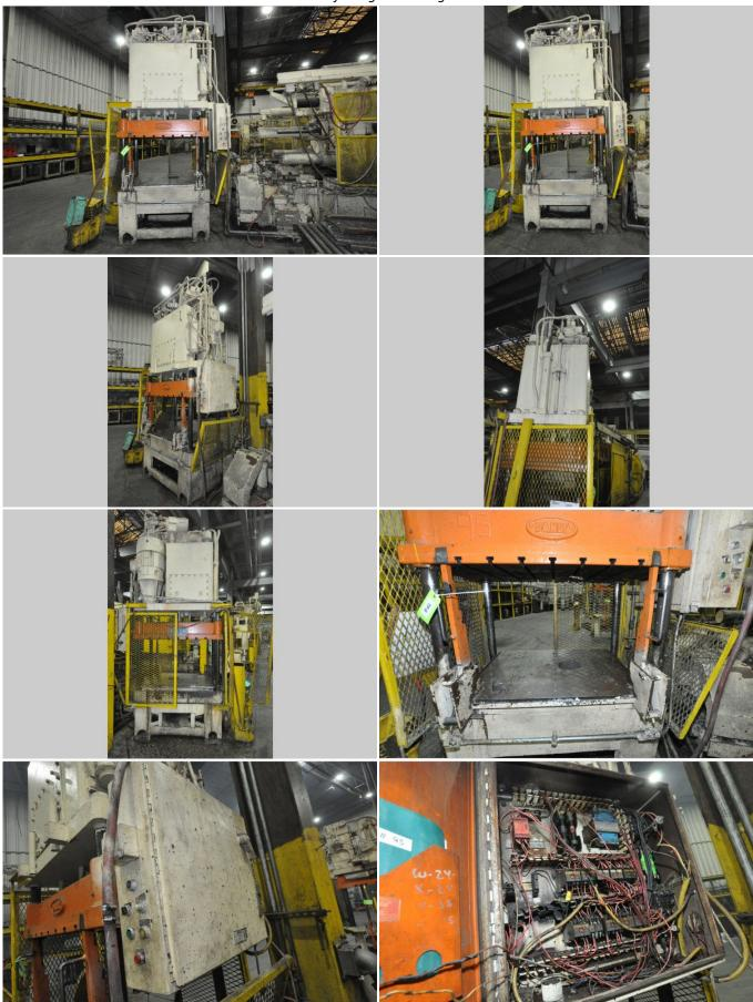
**Description:** Used, Danley Model TP-30-7 30 U.S. Tons Four Column (Post) Vertical Hydraulic Die Casting Trim Press For Sale, Features include: T-Slotted Movable Platten, Drill& Tapped Bed, Dual Pull-Out Bar Operation, Top Mounted Hydraulics, , , Relay Controls, Second Hand, DCM-5073
