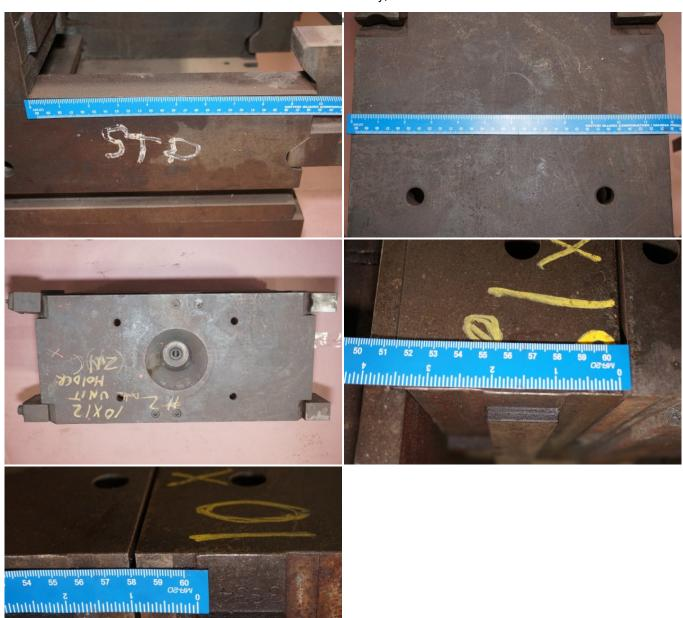
**Description:** Used, DME Model DC-1012-Z 1012 Inch Standard Duty, Double Unit, Hot Chamber Zinc master unit die holder For Sale, Features include: Quick Die Change, Standard Duty Design, Double Holder - holds two inserts, Hot Chamber Configuration, Ships from stock from our Waukegan warehouse, , Controls, Second Hand, DCM-4720
