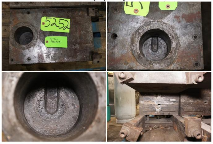
**Description:** Used, DME Model DCS-1012-A 1012 Inch Standard Duty, Single Unit, Cold Chamber Aluminum master unit die holder For Sale, Features include: Quick Die Change System For Die Casting - Modular Unit Design - MUD, DME Standard Duty Design, Single Unit Holder - Holds one set of inserts, Cold Chamber Configuration for Cold Chamber Aluminum or Cold Chamber Magnesium Die Casting, , , Controls, Second Hand, DCM-5252
