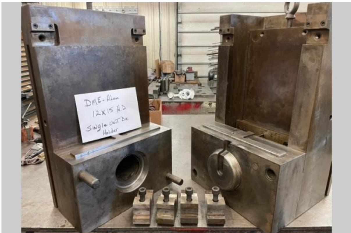
**Description:** Used, DME Model DCS-1215-A-HD 1215 Inch Heavy Duty, Single Unit, Cold Chamber Aluminum master unit die holder For Sale, Features include: Quick Die Change System For Die Casting - Modular Unit Design - MUD, DME Heavy Duty Design, Single Unit Holder - Holds one Set of inserts, Cold Chamber Configuration for Cold Chamber Aluminum or Cold Chamber Magnesium Die Casting, Ships from Stock from our Warehouse, , Controls, Second Hand, DCM-5460
