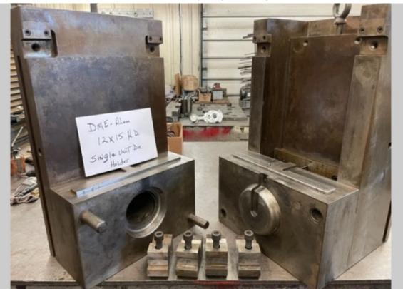
**Description:** Used, DME Model DCS-1215-A-HD 1215 Inch Heavy Duty, Single Unit, Cold Chamber Aluminum master unit die holder For Sale, Features include: Quick Die Change System For Die Casting - Modular Unit Design - MUD, DME Heavy Duty Design, Single Unit Holder - Holds one Set of inserts, Cold Chamber Configuration for Cold Chamber Aluminum or Cold Chamber Magnesium Die Casting, Ships from Stock from our Warehouse, , Controls, Second Hand, DCM-5460
