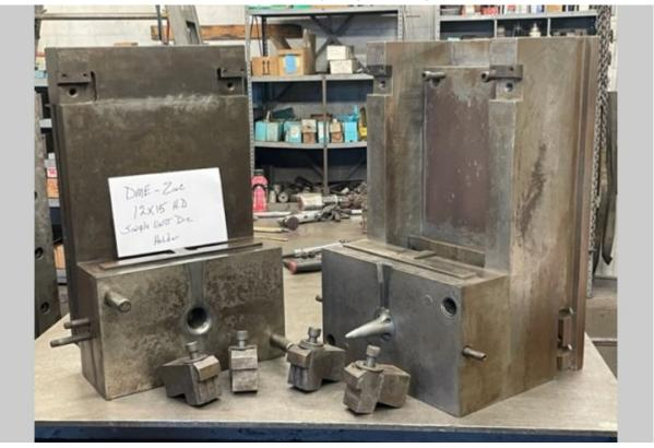
**Description:** Used, DME Model DCS-1215-Z-HD 1215 Inch Heavy Duty, Single Unit, Hot Chamber Zinc master unit die holder For Sale, Features include: Quick Die Change - MUD, Heavy Duty Design, Single Unit Holder - holds one insert, Hot Chamber Configuration, Ships from stock from our Waukegan warehouse, , Controls, Second Hand, DCM-5461
