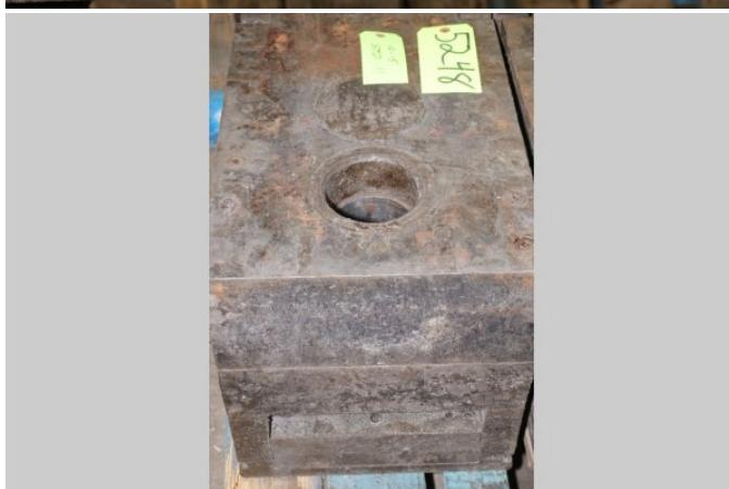
**Description:** Used, DME Model DCS-1215-A 1215 inch Standard Duty, Single Unit, Cold Chamber Aluminum master unit die holder For Sale, Features include: Quick Die Change System For Die Casting - Modular Unit Design - MUD, DME Standard Duty Design, Single Unit Holder - Holds one set of inserts, Cold Chamber Configuration for Cold Chamber Aluminum or Cold Chamber Magnesium Die Casting, , , Controls, Second Hand, DCM-5248
