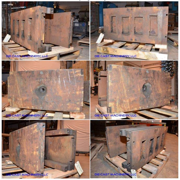
**Description:** Used, DME Model DC-1518-Z 1518 Inch Standard Duty, Double Unit, Hot Chamber Zinc master unit die holder For Sale, Features include: Quick Die Change, Standard Duty Design, Holds up to two (2) Cavity Inserts, Hot Chamber Configuration, Ships from stock from our Waukegan warehouse, , Controls, Second Hand, DCM-3485
