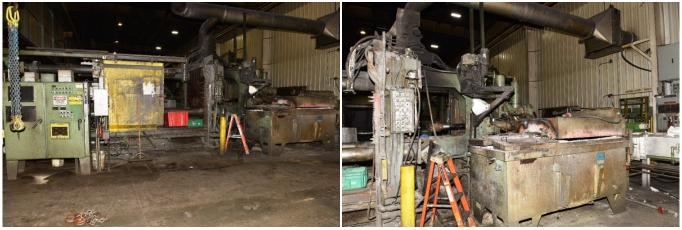
**Description:** Used, Ex-Cell-O B&T Model DC-850 850 Ton Horizontal Cold Chamber Aluminum High Pressure Die Casting Machine For Sale, Features include: Allen Bradley SLC 5/03 Controls with PanelView 600 HMI, Twin Cylinder Hydraulic Bumper Plate Ejection, Electric Motorized Die Height Adjustment, Trabon Heavy Oil Type Automatic Lubrication System, , , Allen Bradley SLC 5/05 with PanelView 600 HMI Controls, Second Hand, DCM-5643
