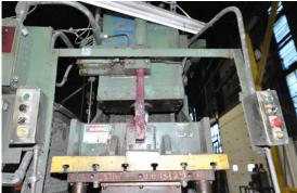
**Description:** Used, Hannifin Press Model OGP-38 38 Ton C-Frame (Gap Frame) Vertical Hydraulic Die Cast Trimming Press For Sale, Features include: T-Slotted Moving and Bed Platens, Two (2) Three Inch Guide Bars Guiding Moving Platen, Soft-Touch Dual Palm Button Operation Push, Air Safety Ratchet Device, Two Auxiliary Side Core/Punch Circuits, , Controls, Second Hand, DCM-4483
