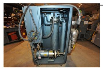
**Description:** Used, HEAT Heat Exchange And Transfer Model KM550-12-483 12 kW Single Zone Portable Hot Oil Process Heater Temperature Control Unit For Sale, Features include: Displays for Process Temperature, Return Temperature and Temperature Difference, Alarms for low fluid pressure, pump rotation, over temperature, Set points for Process, High Alarm, Low Alarm, , , , NEMA 12 Controls, Second Hand, DCM-4093
