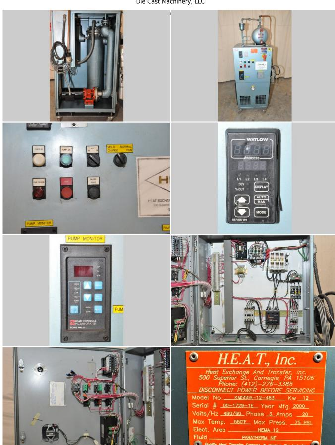
**Description:** Used, HEAT Heat Exchange And Transfer Model KM550A-12-483 12 kW Single Zone Portable Hot Oil Process Heater Temperature Control Unit For Sale, Features include: Displays for Process Temperature, Return Temperature and Temperature Difference, Alarms for low fluid pressure, pump rotation, over temperature, Set points for Process, High Alarm, Low Alarm, , , , NEMA 12 Controls, Second Hand, DCM-4108
