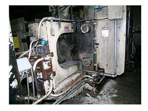
**Description:** Used, HPM Model II-400-A 400 Ton Horizontal Cold Chamber Aluminum/Magnesium Capable High Pressure Die Casting Machine For Sale, Features include: Three Core Circuits, Automatic Operator Side Top Tie Bar Pulling System, Hydrauilc Bumper Platen Ejection System, Hydrauilc Motorized Die Height Adjustment, Trabon Oil Lubrication System, Allen Bradley Relay Controls, Allen Bradley Relay Controls, Second Hand, DCM-1782
