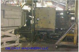
**Description:** Used, HPM Model II-600-A 600 Ton Horizontal Cold Chamber Aluminum High Pressure Die Casting Machine For Sale, Features include: Allen Bradley PLC Controls, Hydraulic Motorized Die Height Adjustment System, Air Safety Ratchet, Hydraulic Bumper Plate Ejection System, Trabon Automatic Linkage Lubrication System (Grease system on Linkage, Oil on Tie Bars), Pre-wired for Automatic Ladle and Automatic Sprayer, Allen Bradley PLC Controls, Second Hand, DCM-3098
