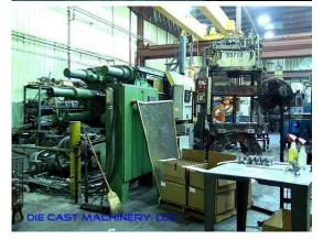
**Description:** Used, Idra Model OL-900-DG 900 Metric Ton Horizontal Cold Chamber Aluminum/Magnesium Capable High Pressure Die Casting Machine For Sale, Features include: Allen Bradley SLC 5/03 Controls, Rimrock 305 Autoladle (new 2006), Rimrock 414 Linear Sprayer (new 2006), ABB IRB 4400 six axis Foundry Plus robot extractor, , , Allen Bradley SLC 5/03 Controls, Second Hand, DCM-1857
