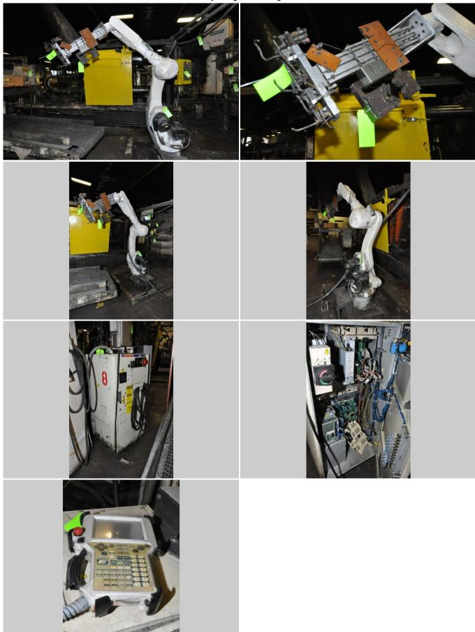
**Description:** Used, Kawasaki Model RS-080N 80 Kilogram Six Axis Foundry Rated Industrial Robot For Sale, Features include: Equipped with a Parts Gripper for Gripping Die Casting Biscuit and also equipped with a Die Lube Spray Package, Fast maneuverability, Heavy Payload Capability, Renowned Kawasaki Parts and Service, Compact Arm Design, , E32F B002 Type E Controls, Second Hand, DCM-4794
