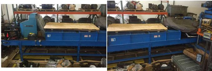
**Description:** Used, Mayfran Model 32-384 32 Inch Wide Steel Hinge type Parts Conveyor with Forced Air Cooling Fans and Tunnel for Die Cast and Foundry Applications For Sale, Features include: Designed with Programmable Start/Stop Allowing Parts to Index Allowing For More Part Time, Forced Air Cooling Tunnel, , , , , Programmable Controls, Second Hand, DCM-4052
