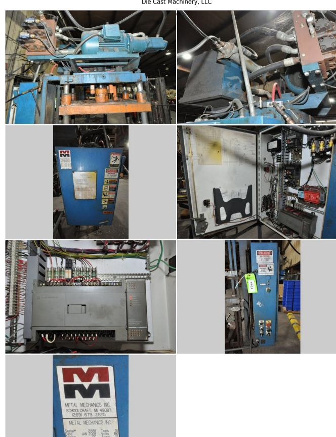
**Description:** Used, Metal Mechanics Model DCT-30 30 U.S. Ton Four Column (Post) Vertical Hydraulic Die Casting Trim Press For Sale, Features include: Air Safety Ratchet Device, Drilled & Taped Bed and Moving Platten, Mechanical Ejection, Dual-Button Operation with Zero-Force Proximity Switch Control, Top Mounted Hydraulics, Allen Bradley SLC 500 Solid State Controls, One (1) Auxiliary Core Circuit, Allen Bradley SLC 500 Solid State Control Controls, Second Hand, DCM-5106
