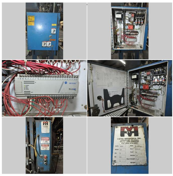
**Description:** Used, Metal Mechanics Model DCT-30 30 U.S. Ton Four Column (Post) Vertical Hydraulic Die Casting Trim Press For Sale, Features include: Air Safety Ratchet Device, Drilled & Taped Bed, T-Slotted Moving Platten, Dual-Button Operation with Zero-Force Proximity Switch Control, Top Mounted Hydraulics, Allen Bradley MicroLogix 1000 Solid State Controls, Mechanical Ejection, Allen Bradley MicroLogix 1000 Solid State Control Controls, Second Hand, DCM-5108
