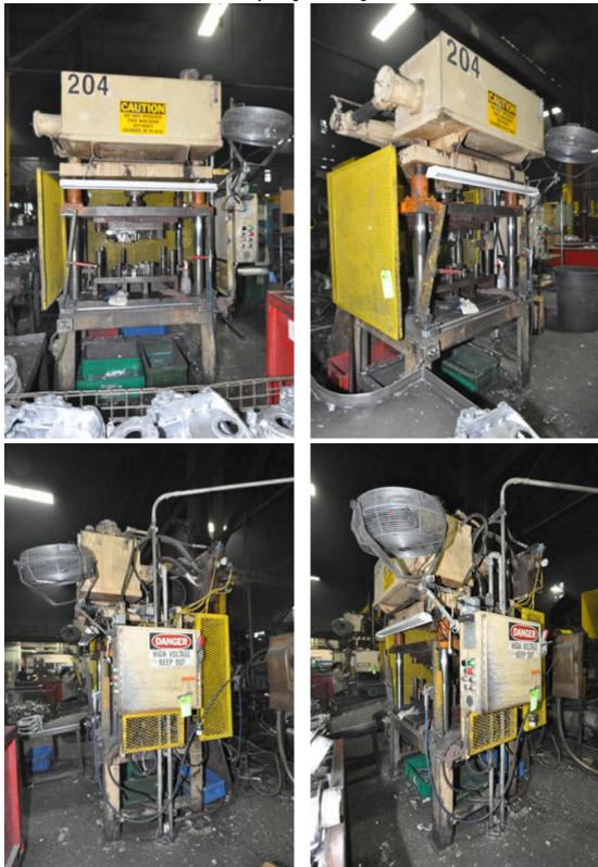
**Description:** Used, Metal Mechanics Model 35 35 Ton Four Column (Post) Vertical Hydraulic Die Casting Trim Press For Sale, Features include: Dual Pull-Out Bar Operation, T-Slotted Bed, Drilled & Tapped Moving Platen, Allen Bradley SLC Controls, Full Electrical and Hydraulic Documents including Schematics, , , Allen Bradley Solid State Controls, Second Hand, DCM-4500
