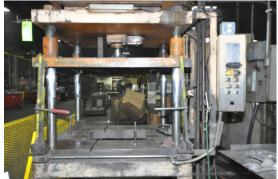
**Description:** Used, Metal Mechanics Model 35 35 Ton Four Column (Post) Vertical Hydraulic Die Casting Trim Press For Sale, Features include: Dual Pull-Out Bar Operation, T-Slotted Bed, Drilled & Tapped Moving Platen, Allen Bradley SLC Controls, Air Safety Ratchet Device, Full Electrical and Hydraulic Documents including Schematics, One (1) Auxiliary Side Core Punch, Allen Bradley Solid State Controls, Second Hand, DCM-4521
