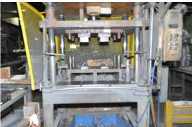
**Description:** Used, Metal Mechanics Model 35 35 Ton Four Column (Post) Vertical Hydraulic Die Casting Trim Press For Sale, Features include: Dual Pull-Out Bar Operation, T-Slotted Bed, Drilled & Tapped Moving Platen, Allen Bradley SLC Controls, Air Safety Ratchet Device, Full Electrical and Hydraulic Documents including Schematics, One (1) Auxiliary Side Core Punch, Allen Bradley Solid State Controls, Second Hand, DCM-4526
