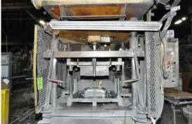
**Description:** Used, Metal Mechanics Model 35 35 Ton Four Column (Post) Vertical Hydraulic Die Casting Trim Press For Sale, Features include: Dual Pull-Out Bar Operation, T-Slotted Bed, Drilled & Tapped Moving Platen, Allen Bradley SLC Controls, Full Electrical and Hydraulic Documents including Schematics, One (1) Auxiliary Side Core Punch, , Allen Bradley Solid State Controls, Second Hand, DCM-4535
