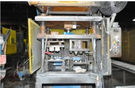
**Description:** Used, Metal Mechanics Model 35 35 Ton Four Column (Post) Vertical Hydraulic Die Casting Trim Press For Sale, Features include: Dual Pull-Out Bar Operation, T-Slotted Bed, Drilled & Tapped Moving Platen, Allen Bradley SLC Controls, Full Electrical and Hydraulic Documents including Schematics, One (1) Auxiliary Side Core Punch, , Allen Bradley Solid State Controls, Second Hand, DCM-4540
