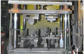
**Description:** Used, Metal Mechanics Model 35 35 Ton Four Column (Post) Vertical Hydraulic Die Casting Trim Press For Sale, Features include: Dual Pull-Out Bar Operation, T-Slotted Bed, Drilled & Tapped Moving Platen, Allen Bradley SLC Controls, Air Safety Ratchet Device, Full Electrical and Hydraulic Documents including Schematics, One (1) Auxiliary Side Core Punch, Allen Bradley Solid State Controls, Second Hand, DCM-4545
