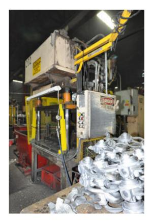
**Description:** Used, Metal Mechanics Model 35 35 Ton Four Column (Post) Vertical Hydraulic Die Casting Trim Press For Sale, Features include: Dual Pull-Out Bar Operation, T-Slotted Bed, Drilled & Tapped Moving Platen, Allen Bradley SLC Controls, Full Electrical and Hydraulic Documents including Schematics, One (1) Auxiliary Side Core Punch, , Allen Bradley Solid State Controls, Second Hand, DCM-4548
