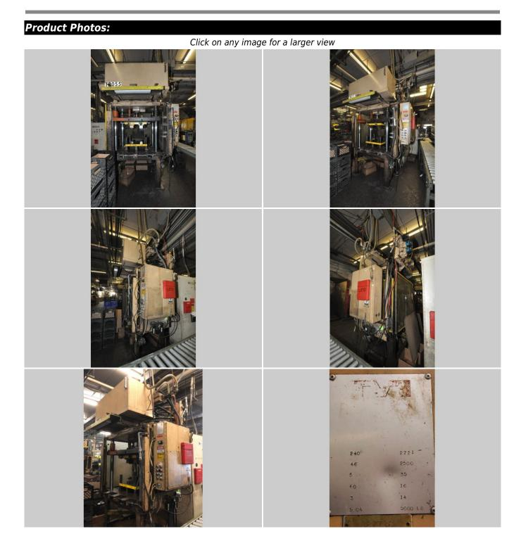
**Description:** Used, Metal Mechanics Model DCT-35 35 U.S. Ton Four Column (Post) Vertical Hydraulic Die Casting Trim Press For Sale, Features include: Air Safety Ratchet Device, T-Slotted Bed & Moving Platen, Allen Bradley Solid State PLC Controls, Dual Palm Button Operation, Light Curtains, One (1) Auxiliary Side Core Punch, Allen Bradley Solid State PLC Controls, Second Hand, DCM-4927
