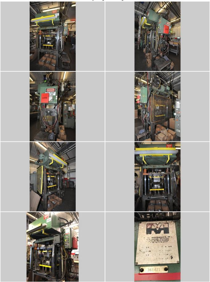
**Description:** Used, Metal Mechanics Model DCT-35 35 U.S. Ton Four Column (Post) Vertical Hydraulic Die Casting Trim Press For Sale, Features include: Air Safety Ratchet Device, T-Slotted Bed & Moving Platen, Allen Bradley Solid State PLC Controls, Dual Palm Button Operation, Light Curtains, One (1) Auxiliary Side Core Punch, Allen Bradley Solid State PLC Controls, Second Hand, DCM-4928
