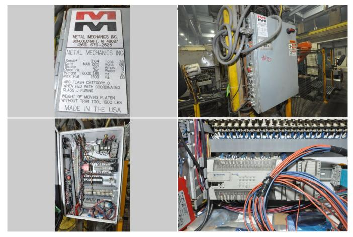
**Description:** Used, Metal Mechanics Model DCT-35 35 U.S. Ton Four Column (Post) Vertical Hydraulic Die Casting Trim Press For Sale, Features include: Air Safety Ratchet Device, Twin Cylinder Hydraulic Bumper Plate Ejection System, T-Slotted Bed & Moving Platen, Allen Bradley Solid State PLC Controls, Palm Button Operation, Light Curtains, One (1) Auxiliary Side Core Punch; Automatic Lubrication System, Allen Bradley Solid State PLC Controls, Second Hand, DCM-5054
