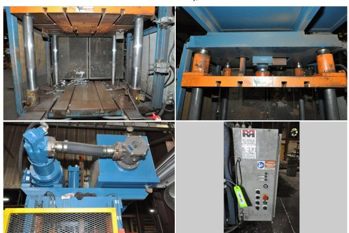
**Description:** Used, Metal Mechanics Model DCT-35 35 U.S. Ton Four Column (Post) Vertical Hydraulic Die Casting Trim Press For Sale, Features include: Air Safety Ratchet Device, T-Slotted Bed & Moving Platen, Proximity Push Buttons, Top Mounted Hydraulics, One (1) Auxiliary Side Core Circuit, Allen BradleyMicrologix 1200 Controls, Second Hand, DCM-5097
