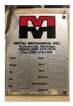
**Description:** Used, Metal Mechanics Model 50 50 Ton Four Column (Post) Vertical Hydraulic Die Casting Trim Press For Sale, Features include: Dual Pull-Out Bar Operation, T-Slotted Platen, Allen Bradley SLC Controls, Full Electrical and Hydraulic Documents including Schematics, Two (2) Auxiliary Hydraulic Side Core Punches, , Allen Bradley Solid State Controls, Second Hand, DCM-4497
