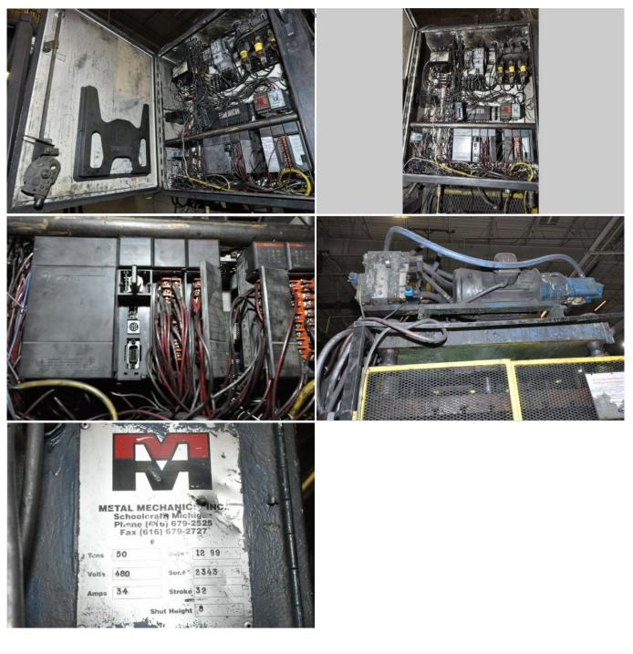
**Description:** Used, Metal Mechanics Model 50 50 Ton Four Column (Post) Vertical Hydraulic Die Casting Trim Press For Sale, Features include: Air Safety Ratchet, Single Palm Button, T-Slotted Bed & Movable Platen, One (1) Auxiliary Hydraulic Side Core Punches, Light Curtains, , Allen Bradley SLC 5/04 Controls, Second Hand, DCM-5211
