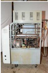
**Description:** Used, Mokon Model H54218-F2 36 kW (18 kW per zone) Dual (two) Zone Portable Hot Oil Process Heater Temperature Control Unit with Cooling Water Circuit For Sale, Features include: HTF 500 Series Mokon Dependability, Water Cooling Circuit, Built-in pump pressure relief valve, Unit on casters for easy movement, Eurotherm Controller, , Eurotherm Controls, Second Hand, DCM-3598
