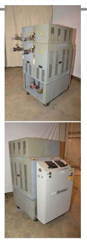
**Description:** Used, Mokon Model H54218-F2 36 kW (18 kW per zone) Dual (two) Zone Portable Hot Oil Process Heater Temperature Control Unit with Cooling Water Circuit For Sale, Features include: HTF 500 Series Mokon Dependability, Water Cooling Circuit, Built-in pump pressure relief valve, Unit on casters for easy movement, Eurotherm Controller, , Eurotherm Controls, Second Hand, DCM-3600
