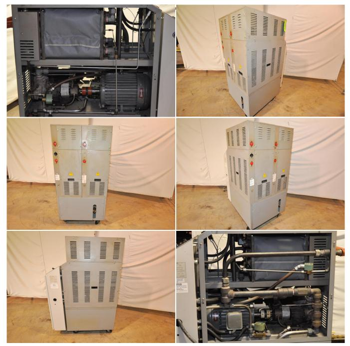
**Description:** Used, Mokon Model H54224Z6 48 KW (24 kw per zone) Dual (two) Zone Portable Hot Oil Process Heater Temperature Control Unit with Cooling Water Circuit For Sale, Features include: HTF 500 Series Mokon Dependability, Water Cooling Circuit, Built-in pump pressure relief valve, Unit on casters for easy movement, Eurotherm Controls, , Eurotherm Controls, Second Hand, DCM-4134
