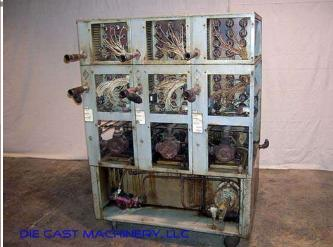
**Description:** Used, Mokon Model H54C24-Y9 72 kW (24 kw per zone) Three Zone Portable Hot Oil Process Heater Temperature Control Unit For Sale, Features include: Self-Contained Three Zone, Unit on Casters for easy movement, Mokon Dependability, , , , Controls, Second Hand, DCM-2411
