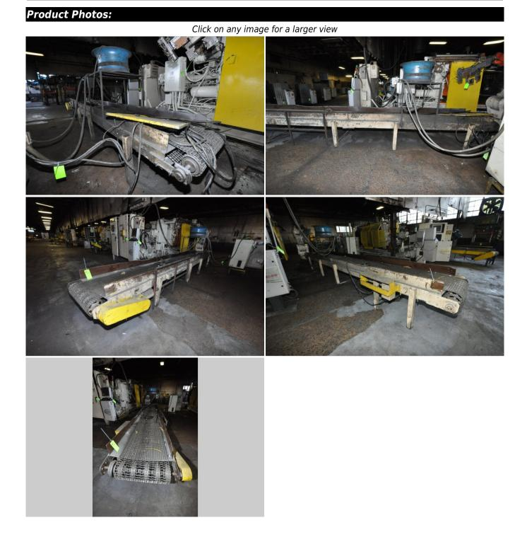
**Description:** Used, PDC Model 24 Inch Wide by 21 foot long Metal Chain Plate Conveyor Belt with Forced Air Cooling Fans and Tunnel for Die Cast and Foundry Applications For Sale, Features include: , , , , , , , Controls, Second Hand, DCM-4841
