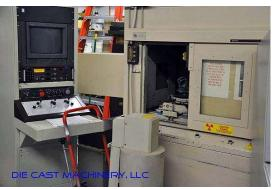
**Description:** One used (second hand) Philips Model MCRS 2000-3 Real Time Industrial X-Ray, Serial Number , 160kv, five Axis Parts Manipulator, New .
