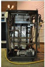
**Description:** Used, Regloplas Model 301DG 72 KW (36 kw per zone) Dual (two) Zone Portable Hot Oil Process Heater Temperature Control Unit For Sale, Features include: Pump with magnetic drive, Leak-free, Separate expansion vessel, Fail-safe circuit in case of heat contactor, , , , RT50 Controls, Second Hand, DCM-3275
