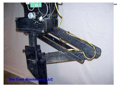
**Description:** Used, Rimrock Model 305 Multi-Link Automatic Ladle for Non-Ferrous Aluminum and Brass Die Casting and Foundry Operations For Sale, Features include: Compact Size, Automatic Pour Back feature, Simple Mechanism, interchangeable parts with other, Works on either operators or helpers side of machine, Excellent Adjustability, , Controls, Second Hand, DCM-1021
