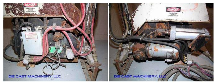
**Description:** Used, Rimrock Model 310 Multi-Link Automatic Reciprocating Die Lubrication Sprayer for Die Casting and Foundry Operations For Sale, Features include: Rimrock, Easy to Program via Teach Pendant Interface, Adjustable Speeds, Positions, Timers and Functions, Uses Rimrock Standard or Picture Frame Sprayer Manifolds with 025 or 026 Nozzles, , , Controls, Second Hand, DCM-1028
