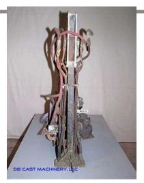
**Description:** Used, Rimrock Model 310 Multi-Link Automatic Reciprocating Die Lubrication Sprayer for Die Casting and Foundry Operations For Sale, Features include: Rimrock, Easy to Program via Teach Pendant Interface, Adjustable Speeds, Positions, Timers and Functions, Uses Rimrock Standard or Picture Frame Sprayer Manifolds with 025 or 026 Nozzles, , , Controls, Second Hand, DCM-1029
