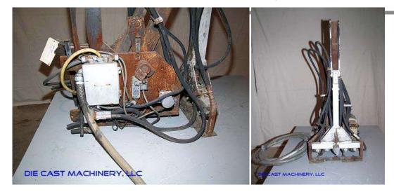
**Description:** Used, Rimrock Model 310 Multi-Link Automatic Reciprocating Die Lubrication Sprayer for Die Casting and Foundry Operations For Sale, Features include: Rimrock , Easy to Program via Teach Pendant Interface, Adjustable Speeds, Positions, Timers and Functions, Uses Rimrock Standard or Picture Frame Sprayer Manifolds with 025 or 026 Nozzles, , , Controls, Second Hand, DCM-1031
