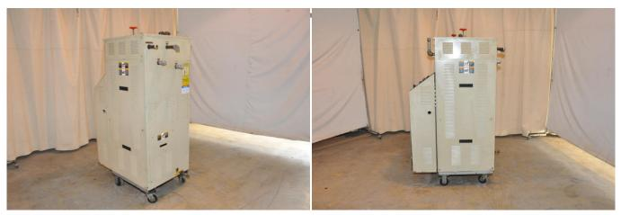
**Description:** Used, Sterlco Model M2A 9016-J1 12 KW Single Zone Portable Hot Oil Process Heater Temperature Control Unit with Cooling Water Circuit For Sale, Features include: M2A Microprocessor Controls, Alarms for low fluid pressure, pump rotation, over temperature, Set points for Process, High Alarm, Low Alarm, Displays for Process Temperature, Return Temperature and Temperature Difference, Water Cooling Circuit, M2A Controls, Second Hand, DCM-4374
