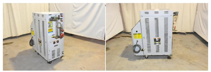
**Description:** Used, Sterlco Model M2B2016-M1 12 KW Single Zone Portable Hot Oil Process Heater Temperature Control Unit with Cooling Water Circuit For Sale, Features include: M2B Microprocessor Controls, Alarms for low fluid pressure, pump rotation, over temperature, Set points for Process, High Alarm, Low Alarm, Displays for Process Temperature, Return Temperature and Temperature Difference, Water Cooling Circuit, M2B Controls, Second Hand, DCM-4420
